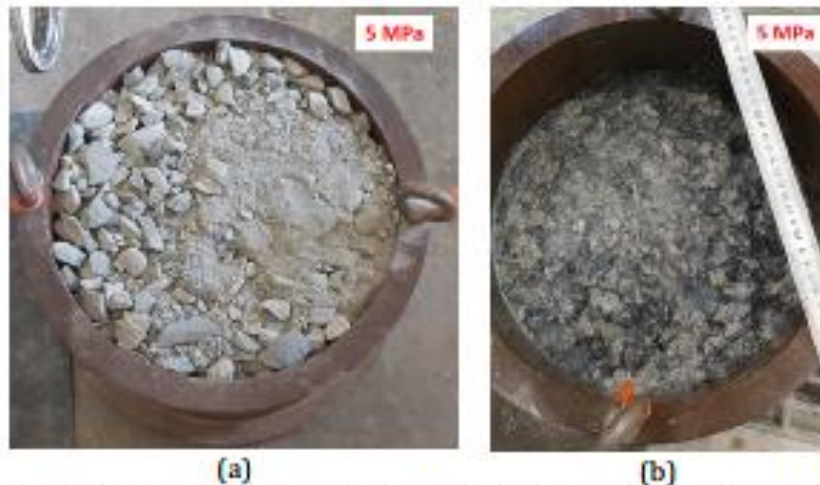
Figure 6 Typical index test specimen: (a) before the test, (b) after the test (wet and consolidated).
