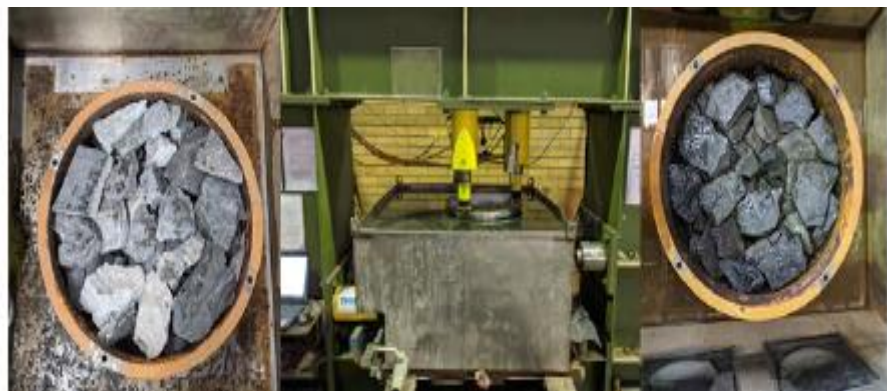
From L-R Saturated induced collapse test before, during and after (using goaf material)
